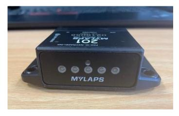
The recommended mounting is on the windscreen in front of the driver or on top of the dash so that the driver can see the unit's lights in their line of sight. If this is not possible, the unit can be mounted anywhere in the vehicle forward of the driver provided that the **unit has a clear view of the sky. It is highly recommended that these units have a secondary tether** if mounted using the 3M Velcro provided as there have been instances of the adhesive failing.
